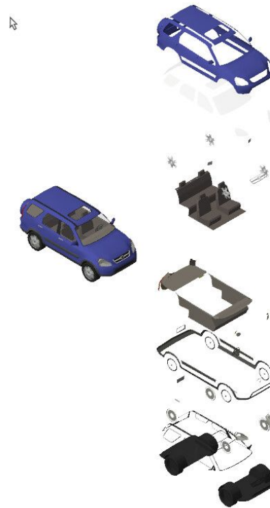
Exploded view showing geometry groups
